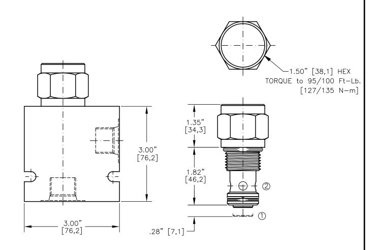
FOR ALUMINUM OR STEEL VALVE HOUSING CONFIGURATIONS SEE PAGE 0-014.1
